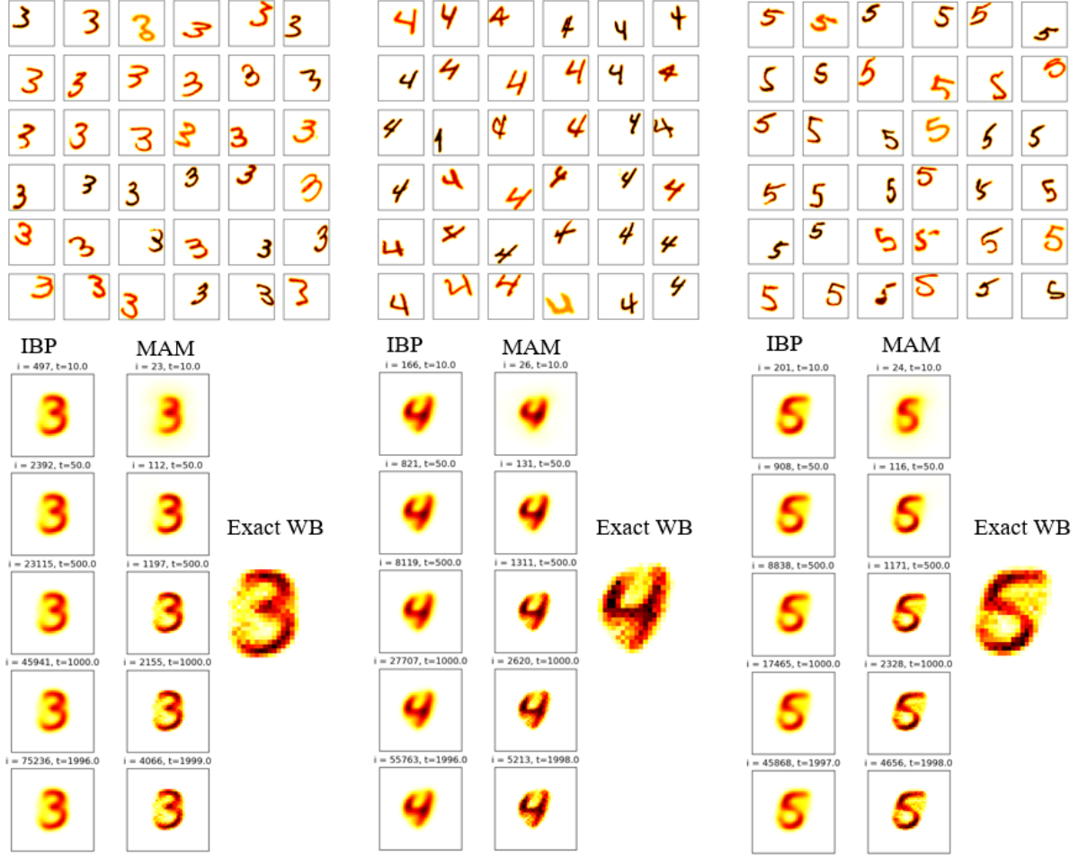
Figure 2.2: (top) For each digit 36 out of the 100 scaled, translated, and rotated images considered for each barycenter. (bottom) Barycenters after t = 10, 50, 500, 1000, 2000 seconds, where the left-hand-side is the IBP evolution of its barycenter approximation, the middle panel is MAM's evolution using 10 CPU and the right-hand-side is a solution computed by applying Gurobi to the LP eq. (2.8).
